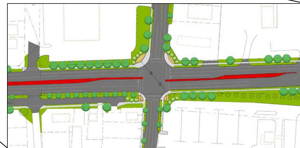
Close up of the Route 21 & 104 intersection showing a colored flush median, trees, and corner treatments.
