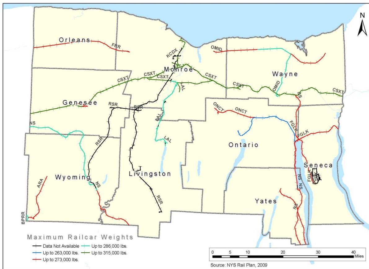
Figure 3.26 Maximum Allowable Railcar Weights
