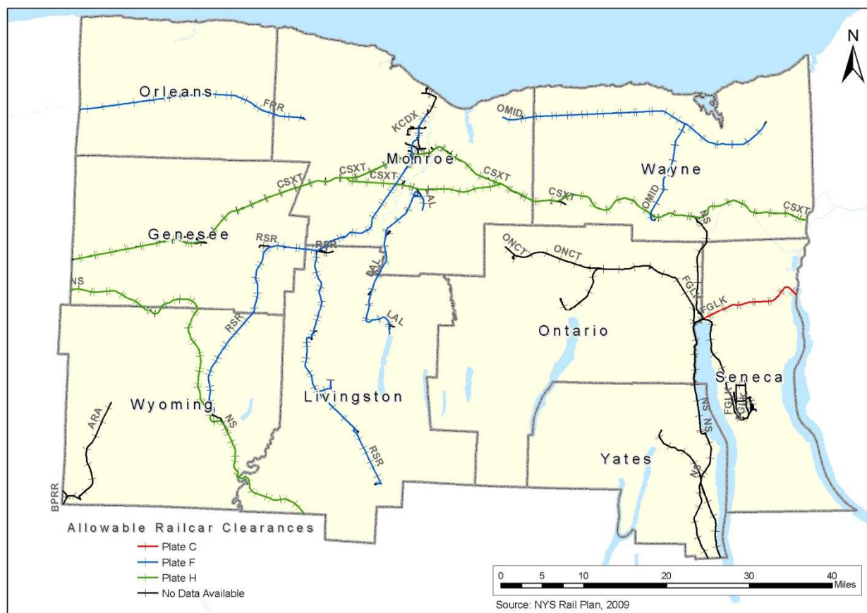
Figure 3.27 Maximum Allowable Railcar Clearances
