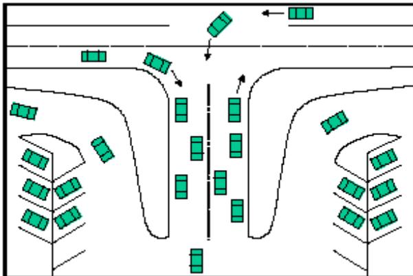
Adequate throat length allows stacking, or queuing, to occur on site. This reduces driver confusion, traffic problems, and unsafe conditions.
