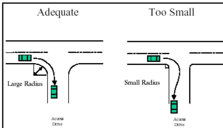
A longer turn radius creates a more rounded corner. This allows the vehicle to enter and exit the driveway more quickly and without encroaching upon traffic in adjacent lanes.
