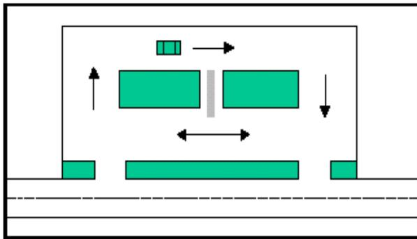
Complete on-site circulation and cross access between adjacent properties allow vehicles to travel between adjacent businesses without having to re-enter the main highway (arterial).
