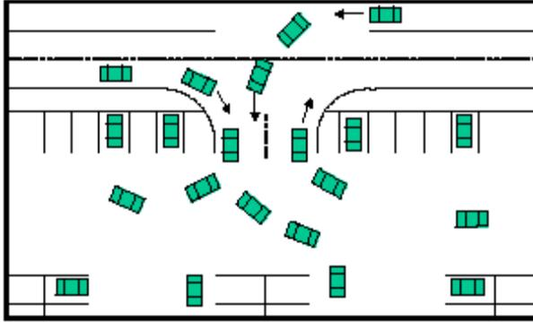
Insufficient throat length and poor site planning can cause unsafe conditions and result in vehicles backing out onto the main highway (arterial), interrupting traffic flow.
