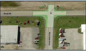
The roadway simulations above show how a dedicated turning lane and signal can be constructed to help alleviated congestion for the existing intersection (top) and a four-way intersection (bottom) if the area is further developed.
