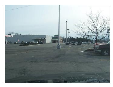
Internal circulation of some plazas indicates poor cross access with non-intersecting roadways and various parking configurations. As shown here the travel lane in this interior parking lot does not align with the travel lane farther ahead. The lack of a coordinated access management between properties, coupled with the expansiveness of pavement and lack of internal landscaping, can contribute to accidents.
