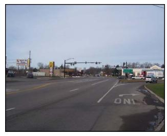
Existing lane striping and access at Route 5 & 63. The short queue length for the turning lanes and multiple curb cuts for the restaurant can be seen at far left.
